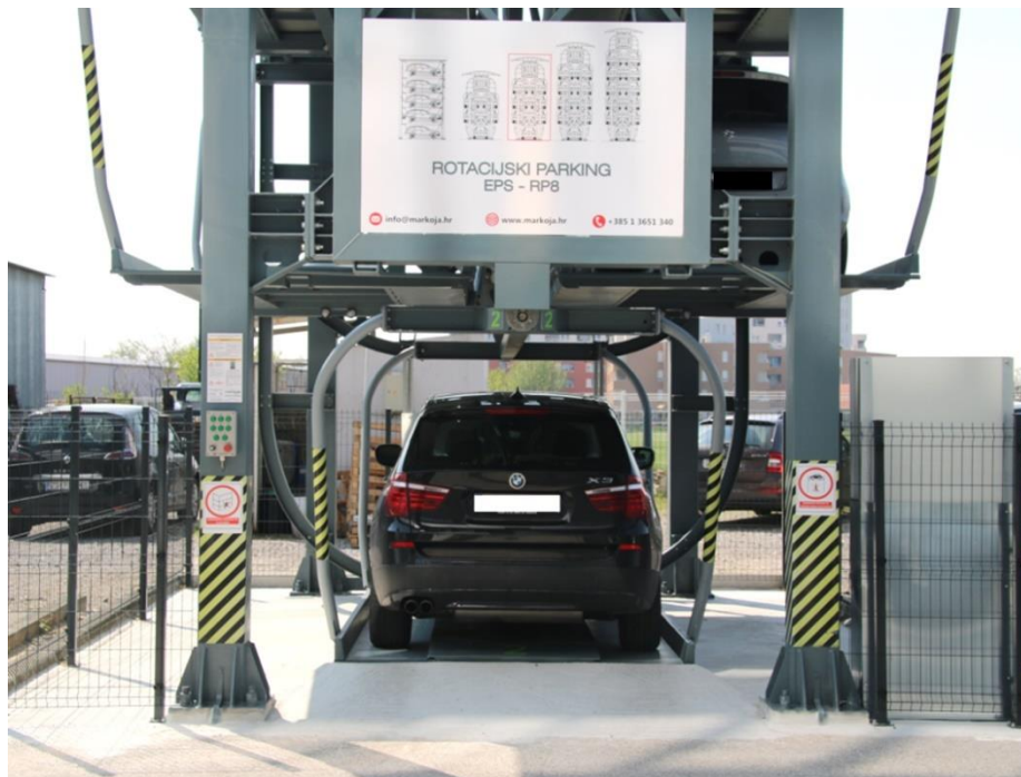
Figure 10: Occupied parking platform at level "0"
