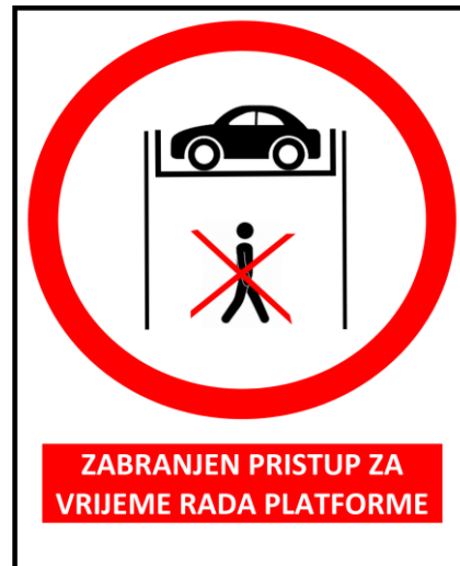
Figure 20: Warning sign for forbidden entry during system operation
