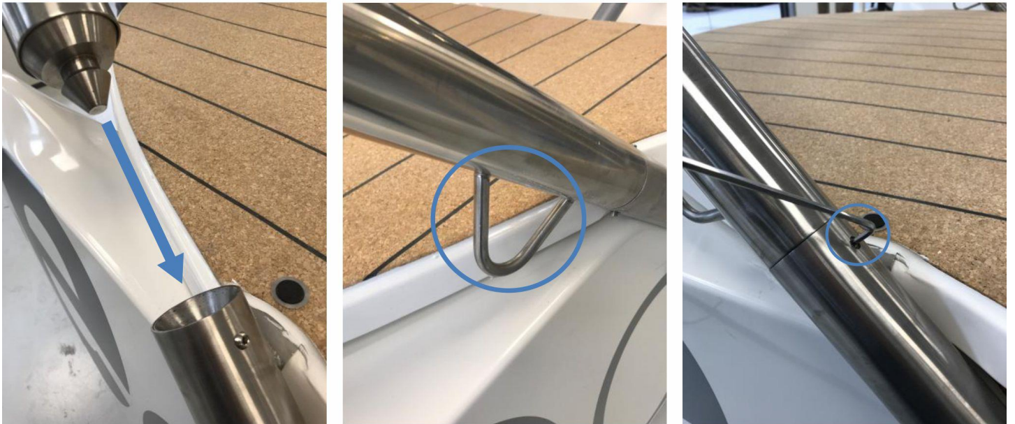
Figure 3: Positioning of the railing.
