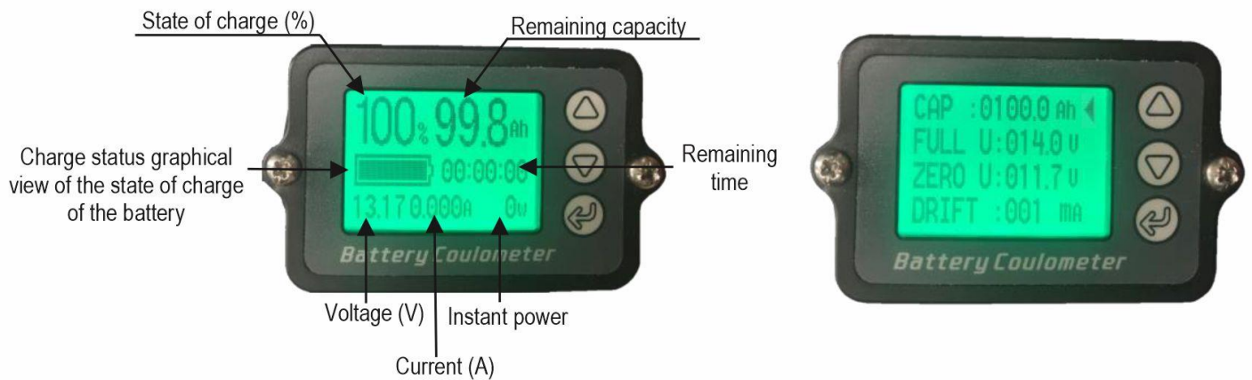
Figure 9: Description of the Coulomb counter interface.
