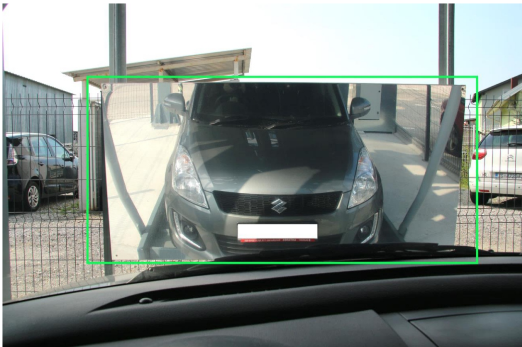
Figure 16: Mirror on the front of the rotary parking for wheel positioning control
