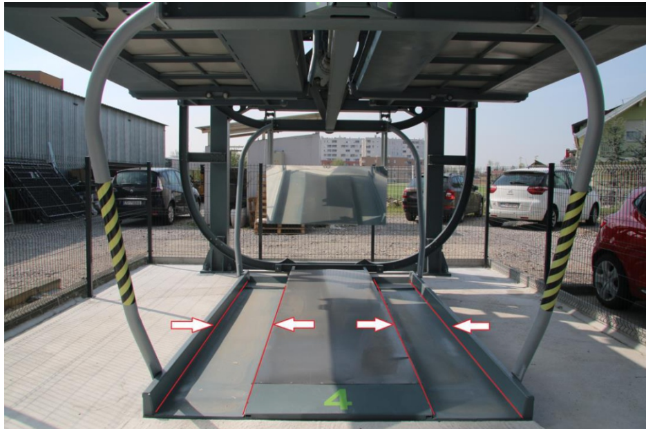
Figure 13: Wheel lanes at the parking platform
