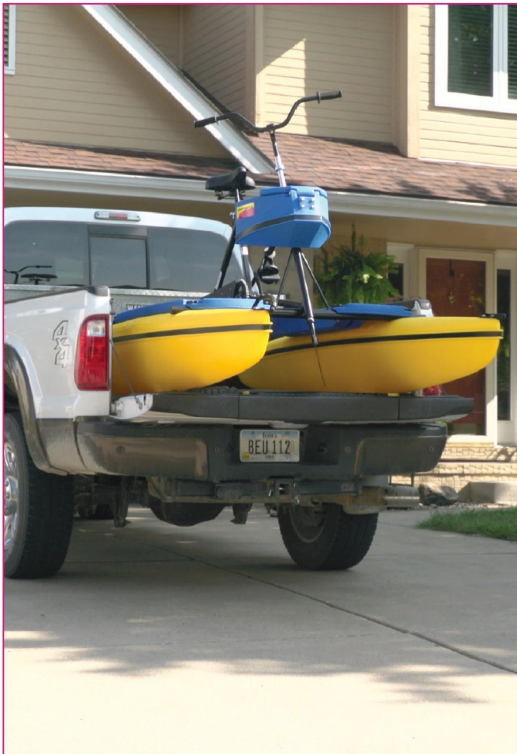
B – FASTEN DOWN THE FRAME OF THE HYDROBIKE TO THE FRAME OF YOUR VEHICLE WITH APPROPRIATE TIE DOWNS.
