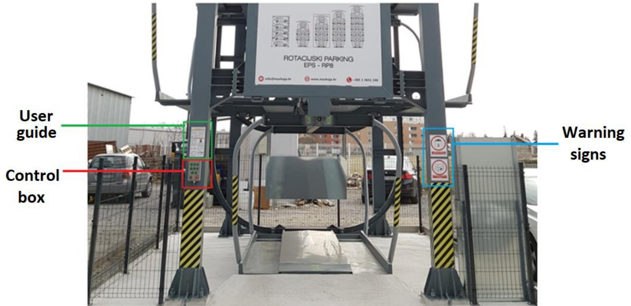
Figure 1: Operation manual and warning signs on the access side of the rotating parking system
