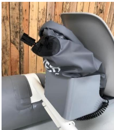
Figure 6: Installing and removing the waterproof bag of the battery.
