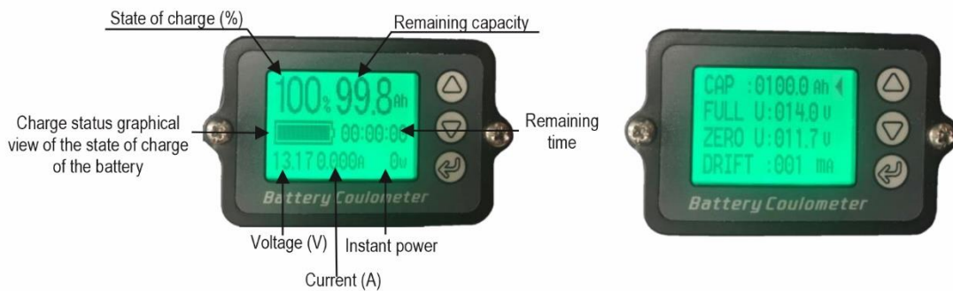
Figure 9: Description of the Coulomb counter interface.
