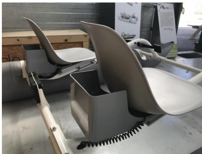
Figure 5: Battery box placement.
